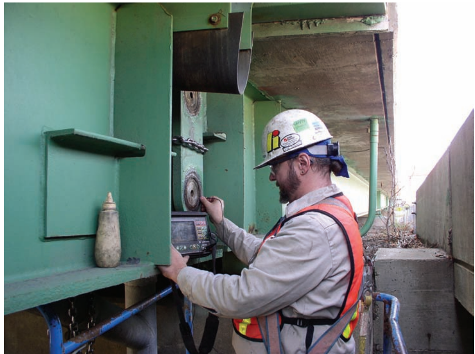
Figure 8.4.17 Ultrasonic Testing of a Pin
